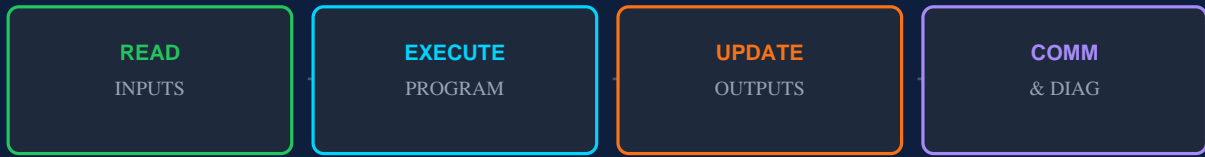
Figure 1.2 PLC Deterministic Scan Cycle (100ms typical)
