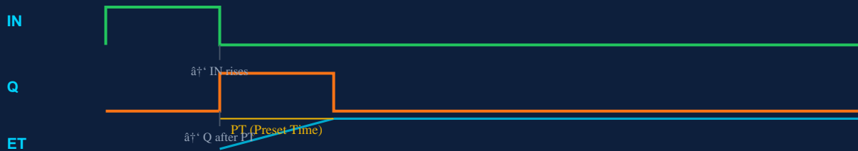
Figure 3.1 “TON (On-Delay Timer) Timing Diagram
